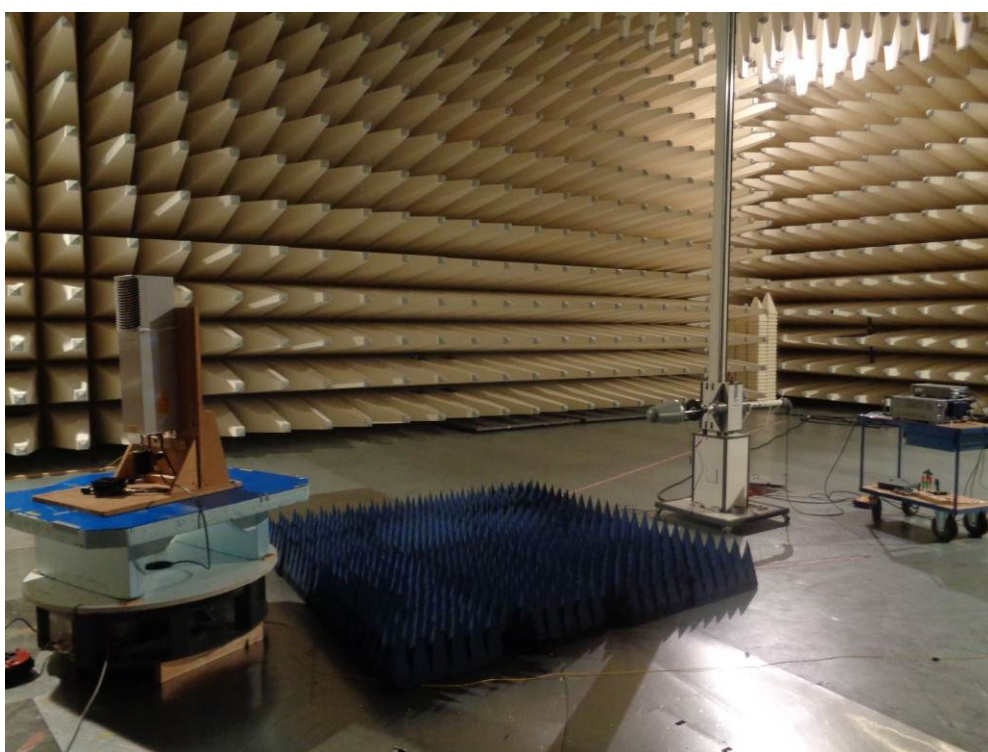
picture 8.4: Test setup: Field Strength Emission >1 GHz @3m in the SAC
