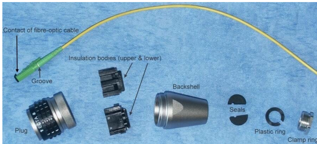
figure 3-15 Protective-plug assembly
