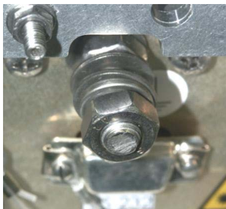
figure 4-6 Grounding bolt with loosened hex nut (left) and schematic view (right)
