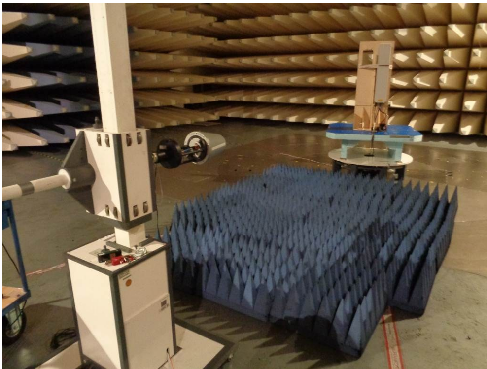
picture 8.3: Test setup: Field Strength Emission 1 - 18 GHz @3m in the SAC
