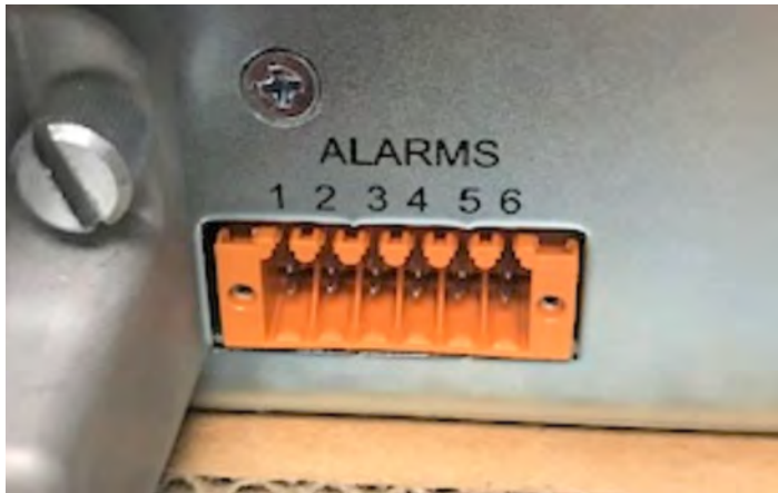
Alarm port on WCS back panel
