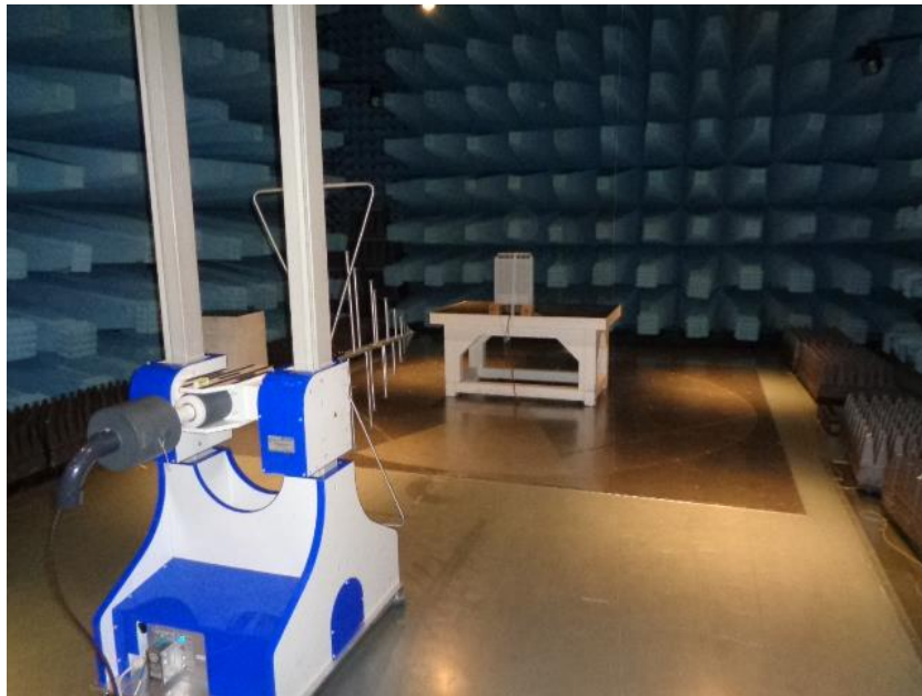
Figure 9.1-3: Radiated emissions set-up for frequencies below 1 GHz
