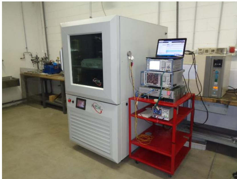
Figure 9.1-2: Antenna port testing set-up in climatic chamber
