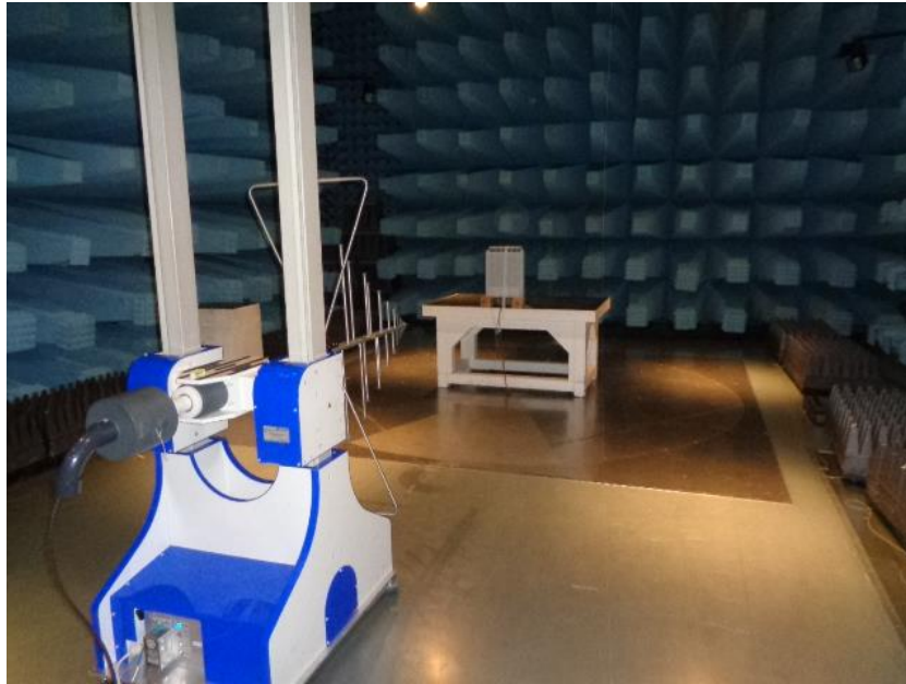
Figure 9.1-3: Radiated emissions set-up for frequencies below 1 GHz
