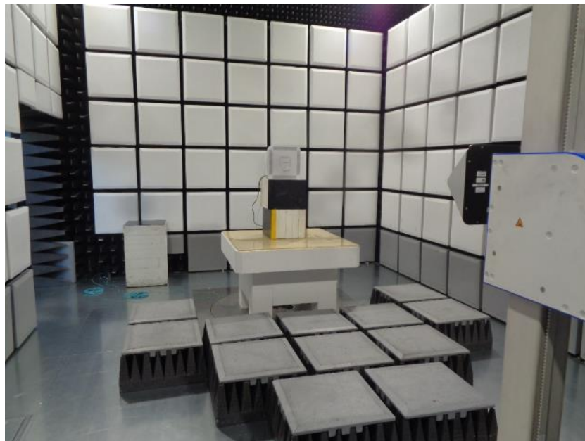
Figure 9.1-4: Radiated emissions set-up for frequencies above 1 GHz
