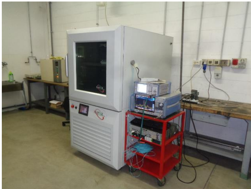
Figure 9.1-2: Antenna port testing set-up in climatic chamber
