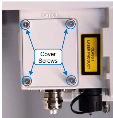
Figure 2-18 Remove optics cover
