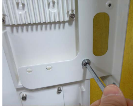
Figure 2-7 Install M6x12 screws and washers for single mount
