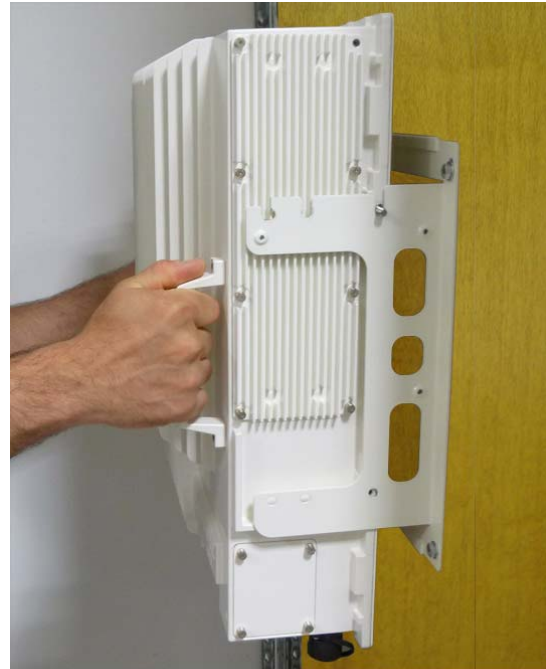
Figure 2-6 Place RU onto wall mounting bracket
