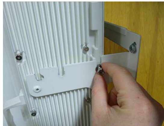
Figure 2-8 Attach M6 nut to threaded pins for single mount
