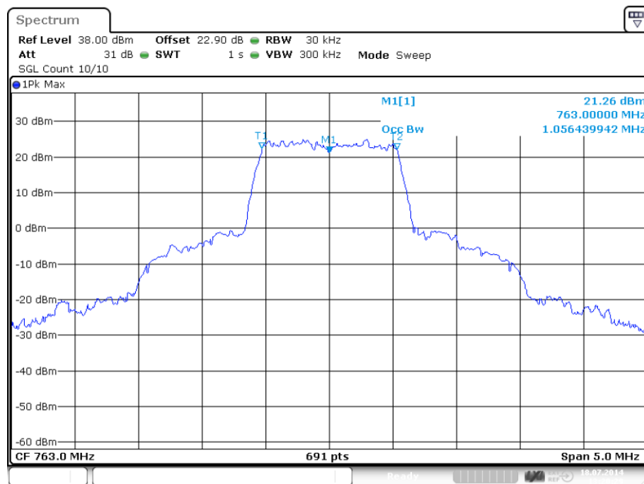
plot 6.3.1.1-#1 Occupied Bandwidth: $90.210, $2.1049; Test results; Downlink; LTE 758 – 768MHz Output
