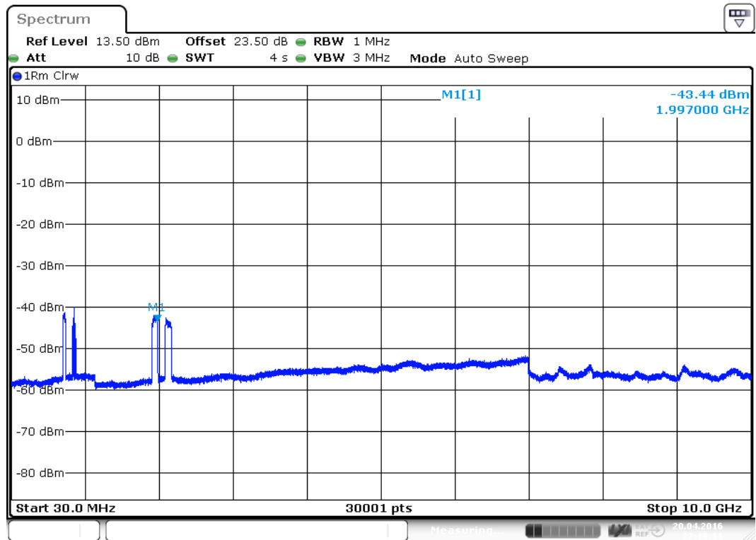
plot 7.3.1.4-#1 Spurious Emissions at Antenna Terminals: §22.917, §2.1051; Test results; Downlink; WCDMA; carrier (881,5MHz) notched
