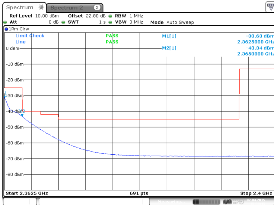
plot 7.3.1.2-#5 Spurious Emissions at Antenna Terminals: §27.53, §2.1051; Test results; Downlink; LTE; 10 MHz signal; 2.3625 GHz – 2.4 GHz; carrier notched
