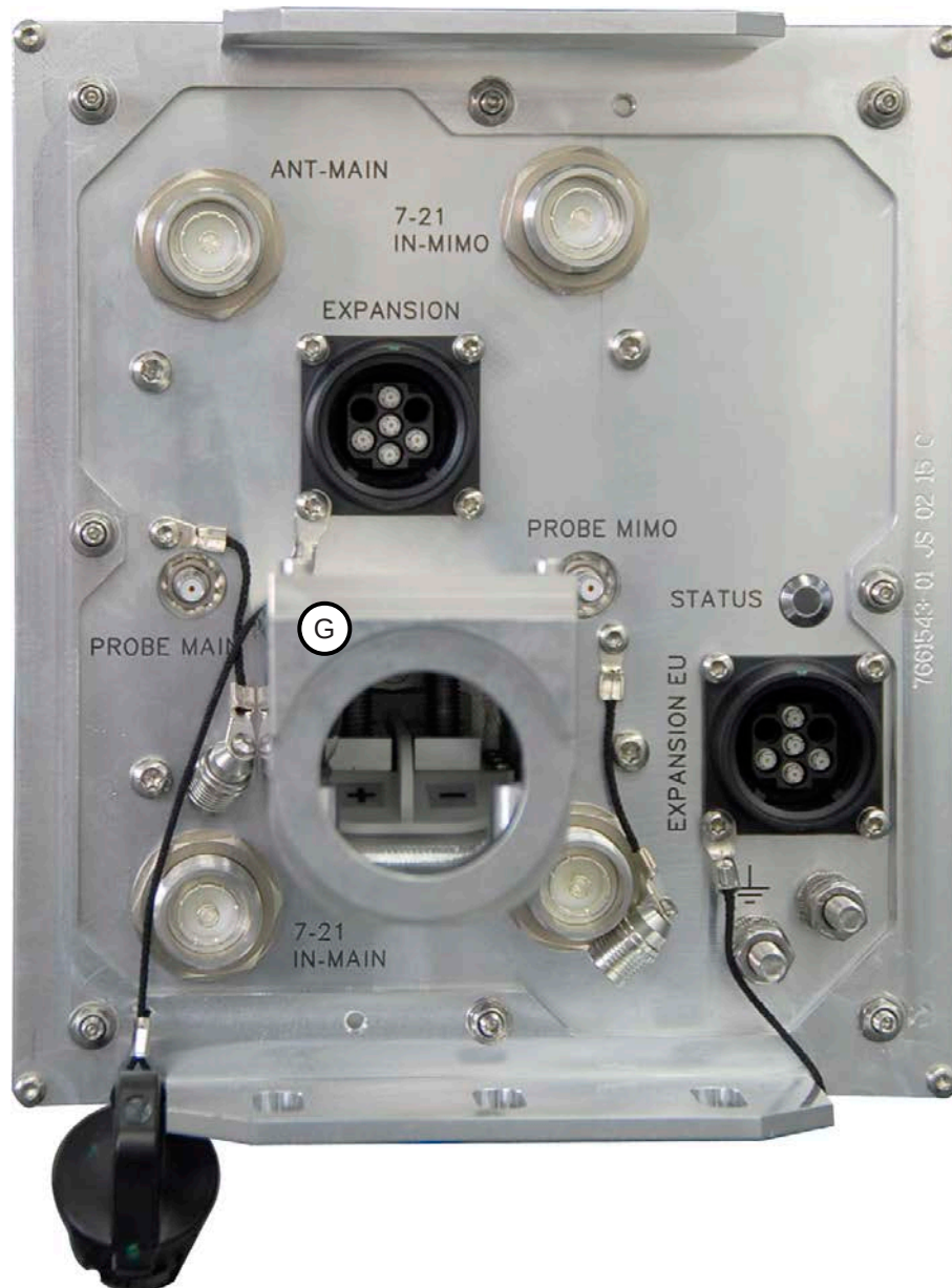
figure 4-12 ION-U EU H 23/23 DC version connector flange
