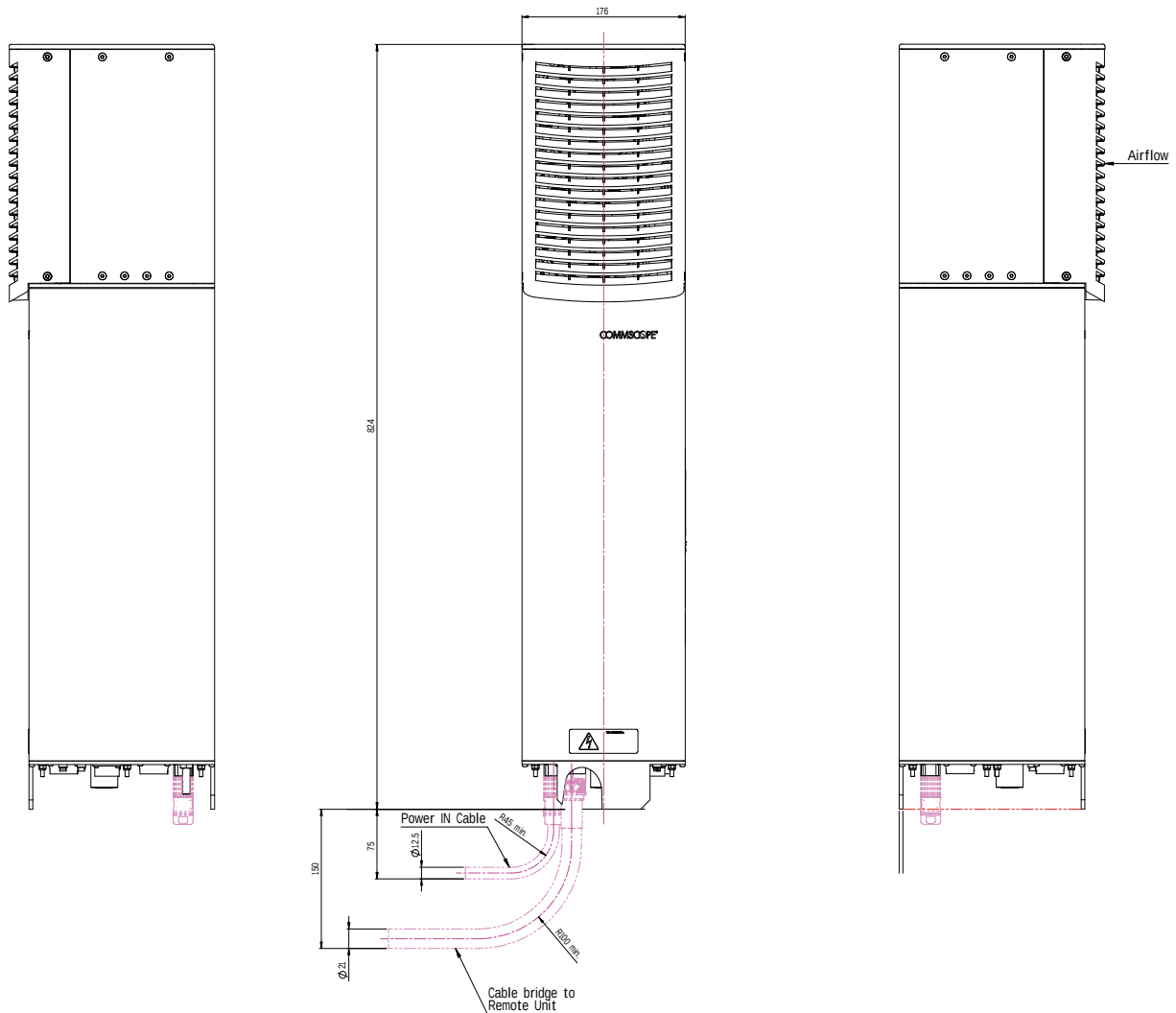
figure 7-1 ION-U EU H 23/23 required space
