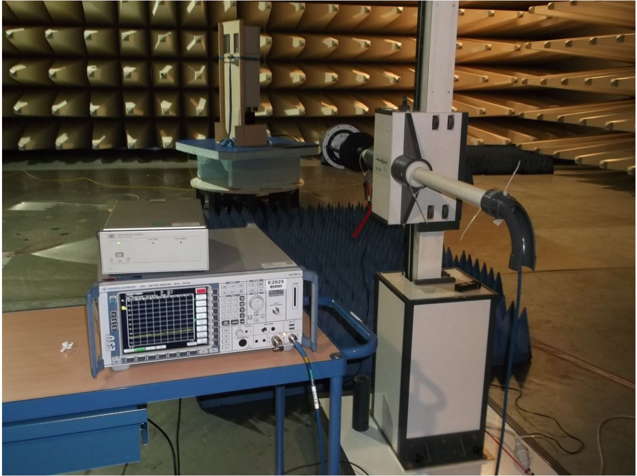
picture 2: Test setup: Field Strength Emission >1 GHz @3m in the SAC
