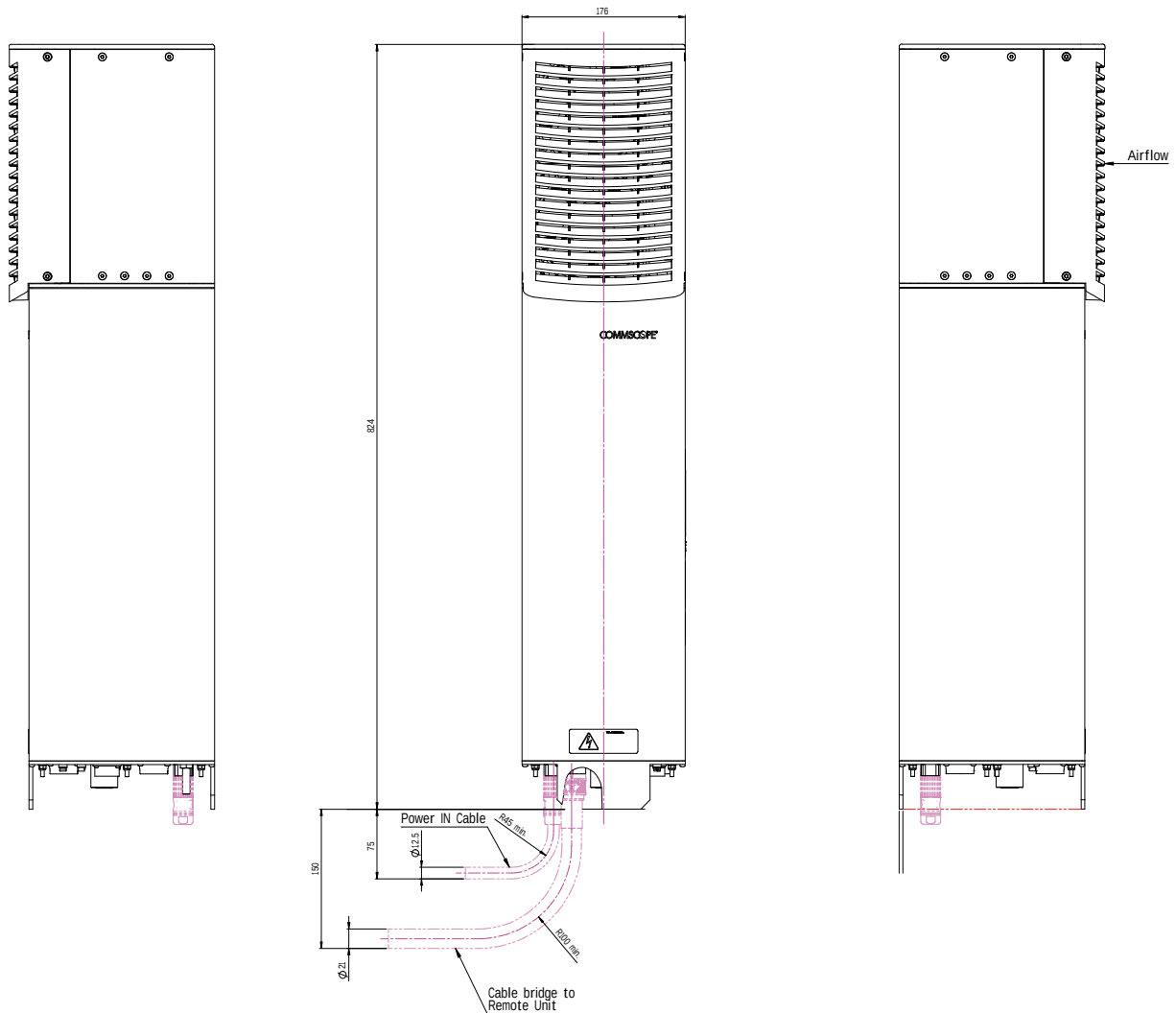
figure 7-1 ION-U EU H 7P/80-85P/17P/19P required space
