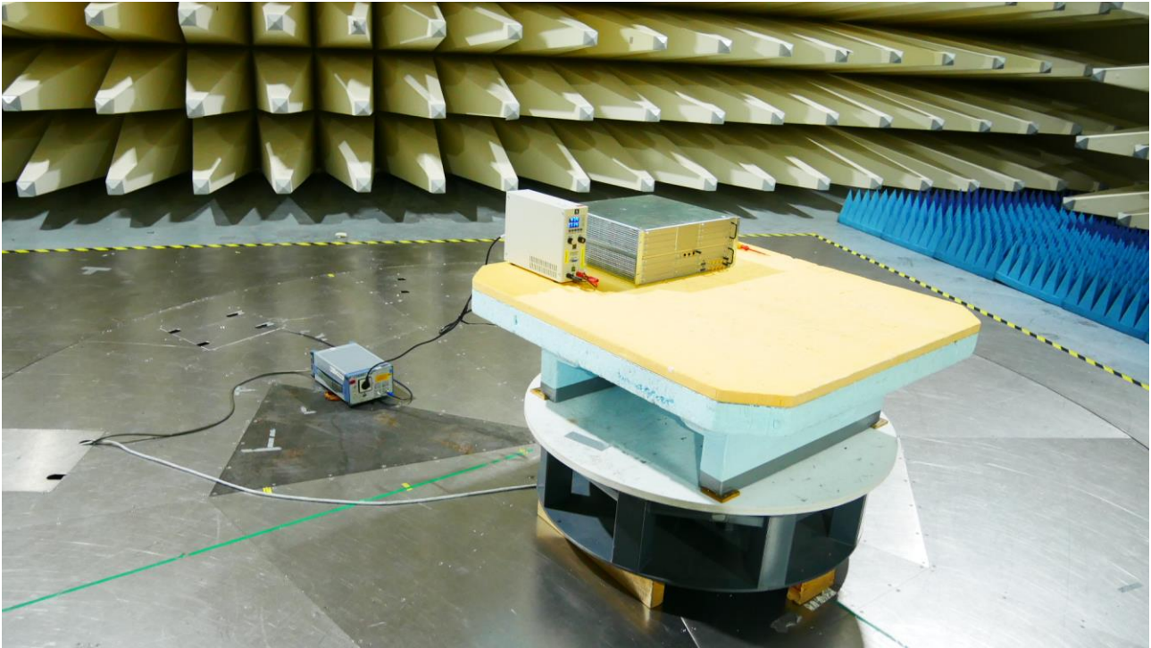
Test setup for AC powerline conducted emissions
