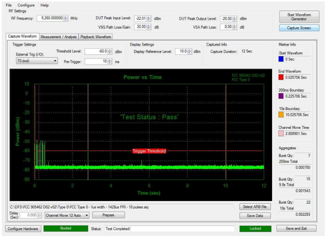
Figure 8.1-1: Channel closing transmission and move time
