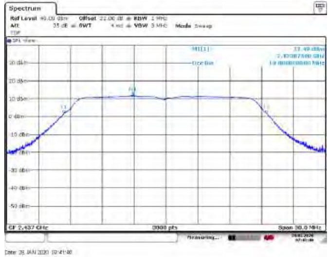
Figure 8.5-17: 99% occupied bandwidth on mid channel, plot
