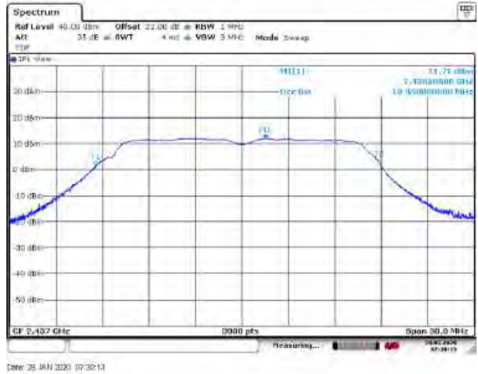
Figure 8.5-11: 99% occupied bandwidth on mid channel, plot
