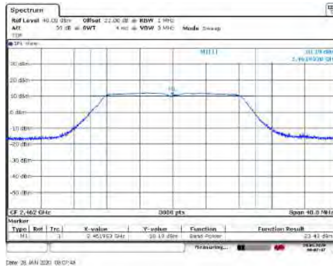
Figure 8.6-9: Output power on high channel, plot
