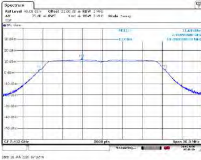
Figure 8.5-16: 99% occupied bandwidth on low channel, plot
