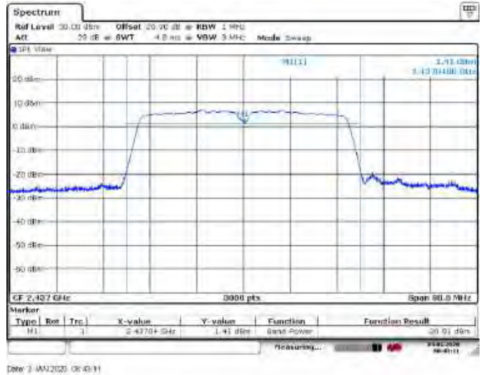
Figure 8.6-11: Output power on mid channel, plot
