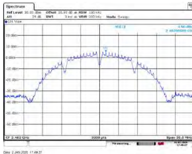
Figure 8.8-3: PSD sample plot on high channel
