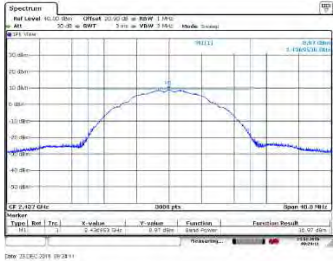
Figure 8.6-2: Output power on mid channel, CCK Modulation
