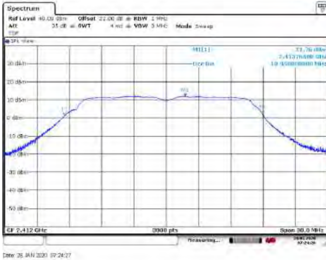
Figure 8.5-10: 99% occupied bandwidth on low channel, plot
