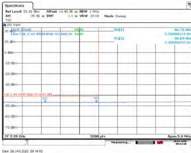
Figure 8.7-22: Restricted Band Edge emissions for low channel, Average
