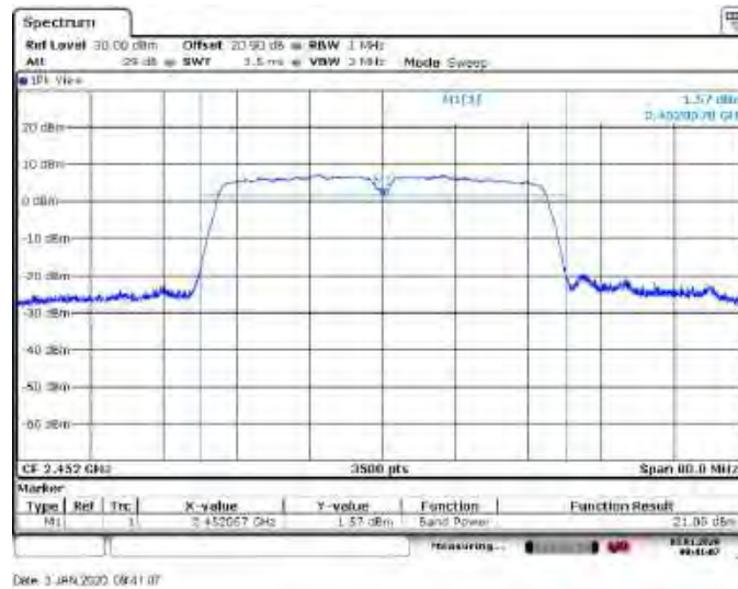
Figure 8.6-12: Output power on high channel, plot
