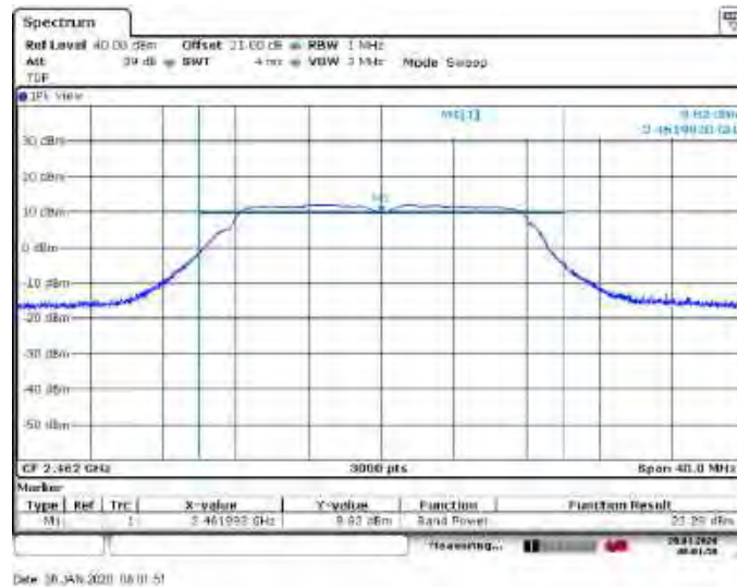
Figure 8.6-6: Output power on high channel, plot
