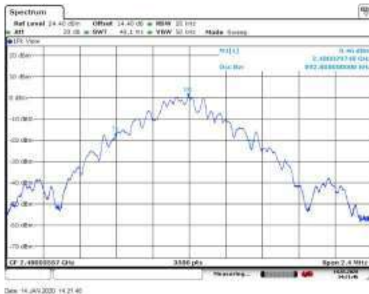
Figure 8.5-6: 99% occupied bandwidth on high channel
