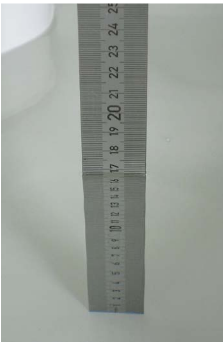
Fig. 15: Liquid depth for IEEE 802.11b body measurements.
