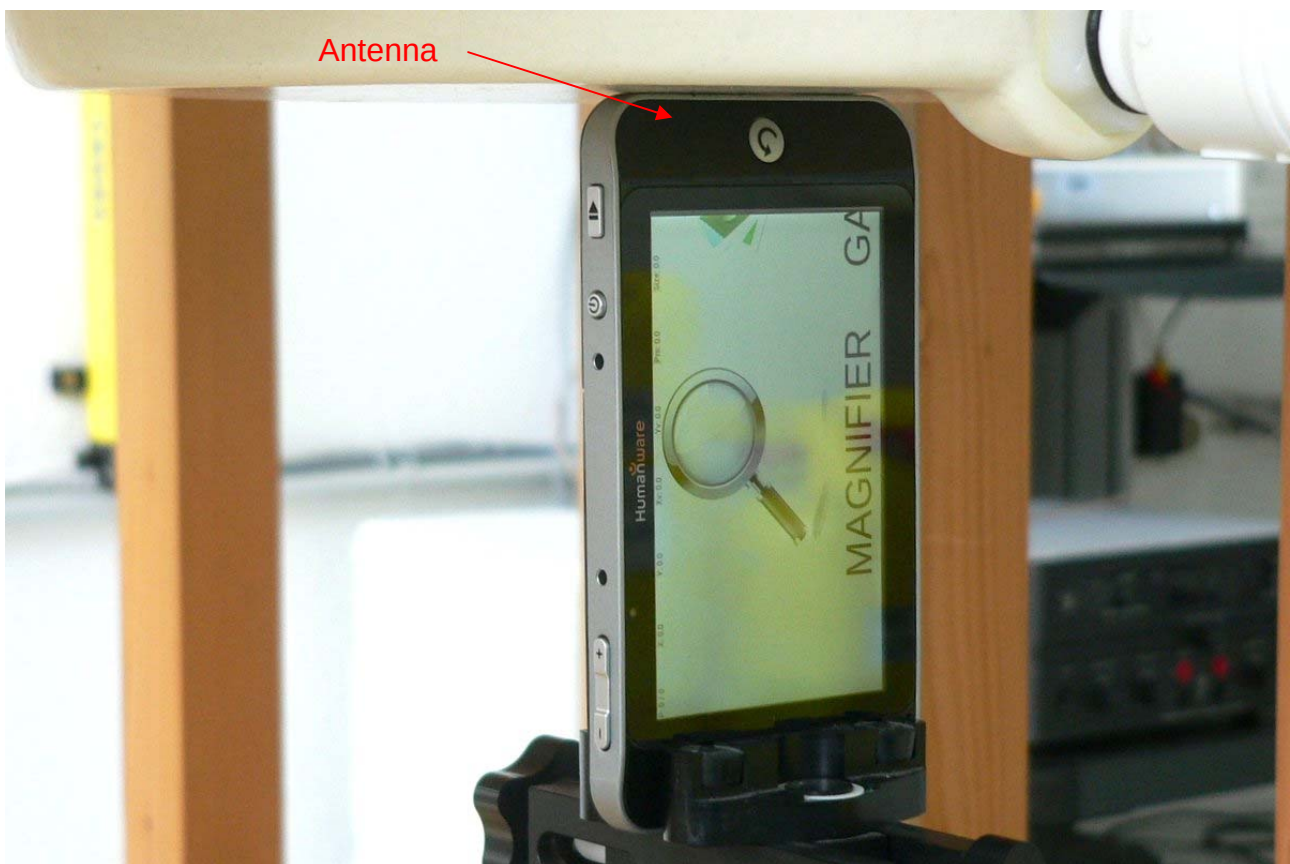
Fig. 13: Body supported configuration, position 4, right edge toward the phantom, gap = 0 mm.
