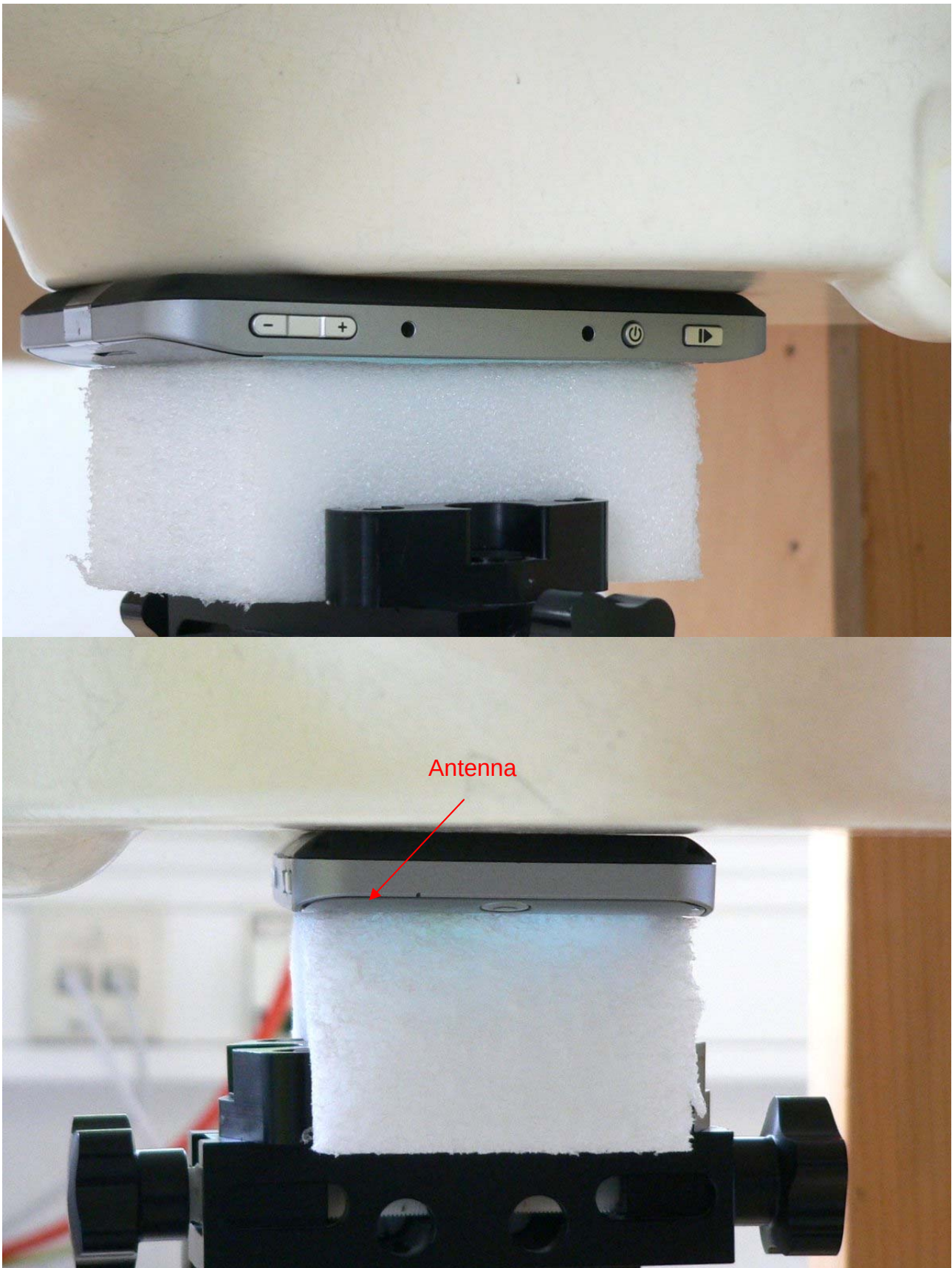
Fig. 11: Body supported configuration, position 2, back side toward the phantom, gap = 0 mm.
