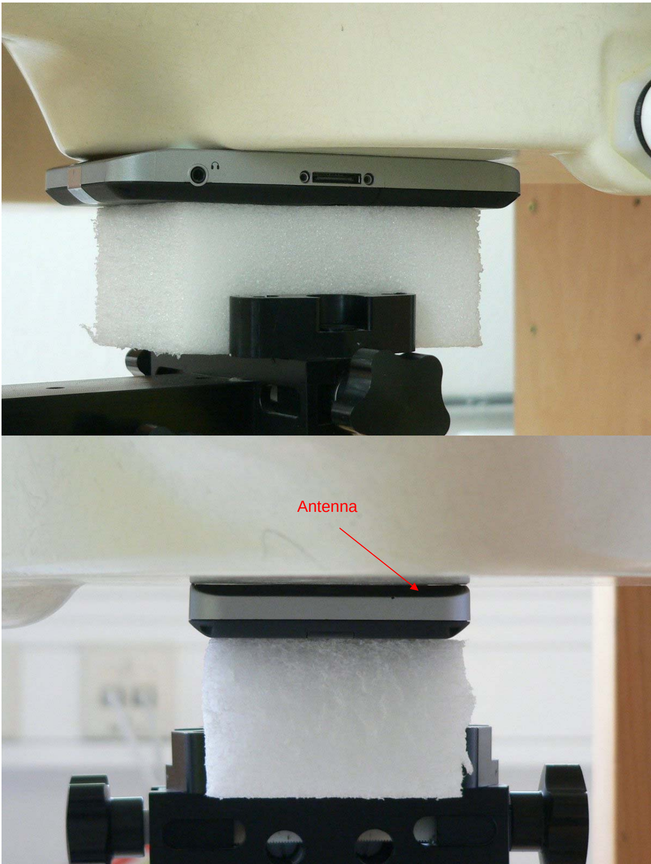
Fig. 10: Body supported configuration, position 1, front side toward the phantom, gap = 0 mm.
