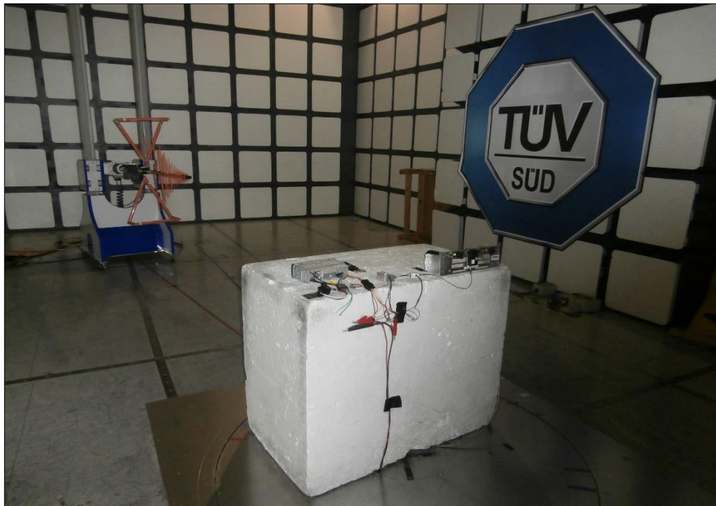
Figure 10 - Test Setup - Below 1 GHz
