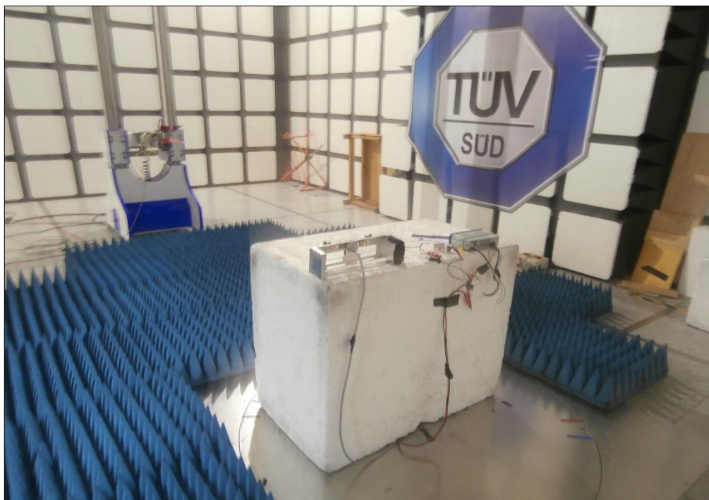
Figure 11 - Test Setup - Above 1 GHz
