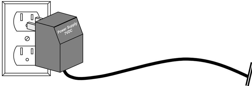
7. Insert the small end of the Power Supply cable into the port labeled "POWER" on the back of Commander FLEX.
