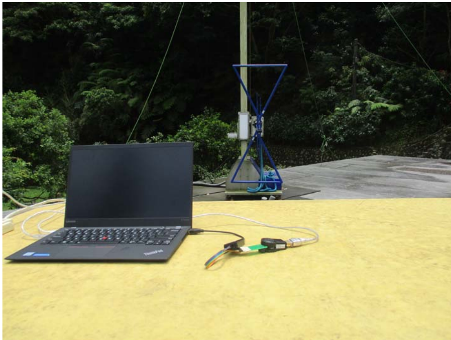
Below 1 GHz (EUT at 0.8m)
