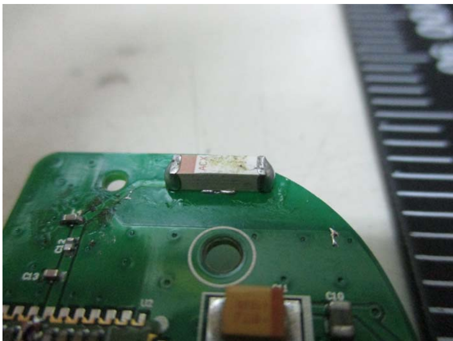
Close Up View of the Chip Antenna
