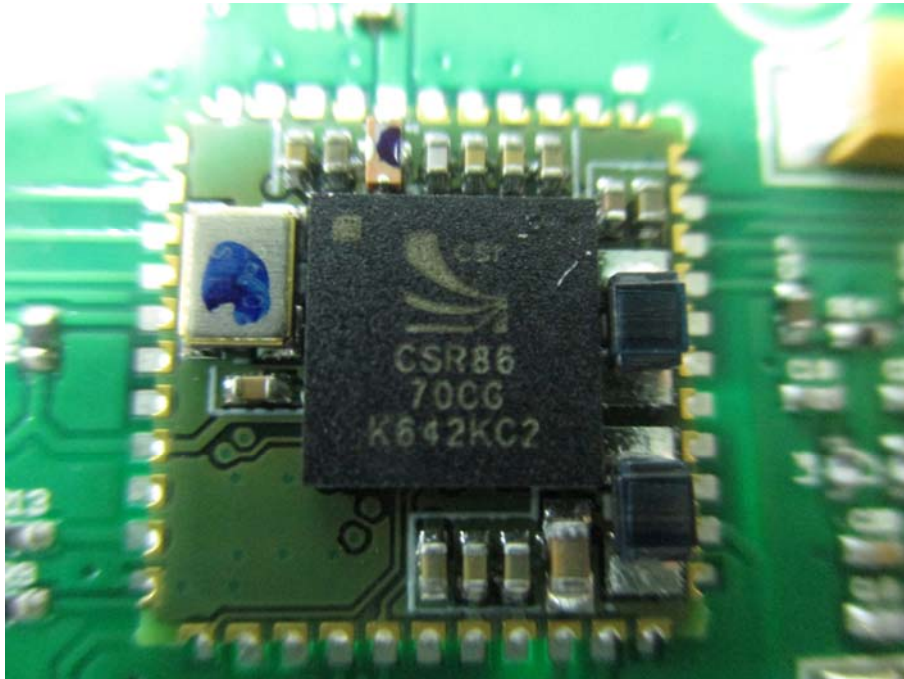
Close Up View of the BT module
