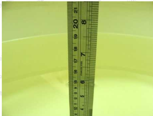
Photo of Liquid Height for Body SAR
