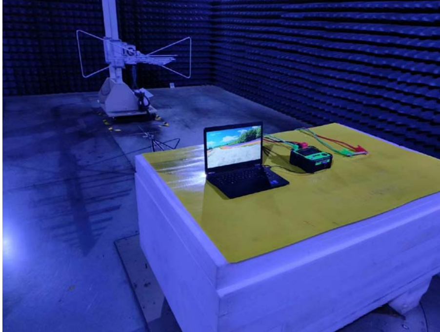
Photo of Radiated Emission Measurement Below 1GHz
