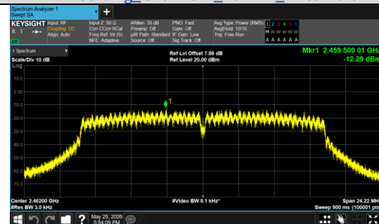
IEEE 802.11g_Channel 11_20MHz_Antenna 0
