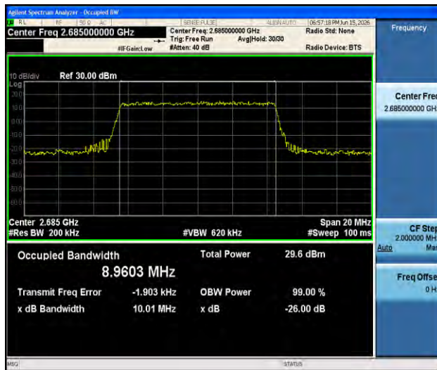
Band41-10MHz-QPSK-41540-50RB#0-PASS
