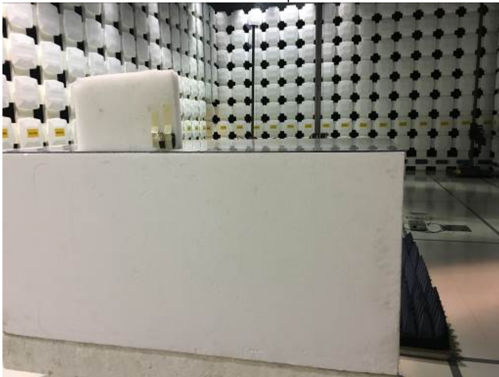
1-18 GHz Test Setup Y-axis
