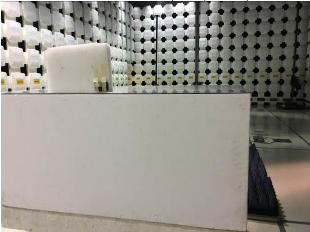
Radiated Emissions Test Setup Y-axis (Worst-case)
