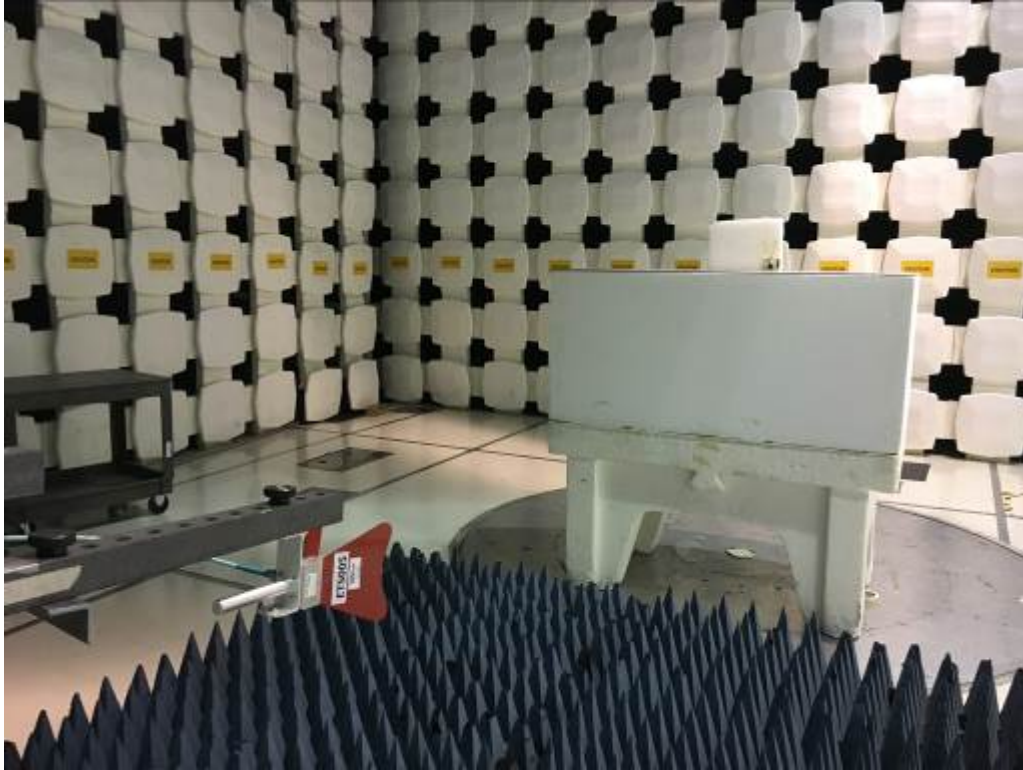
Radiated Emissions Test Setup Y-axis (Worst-case)
