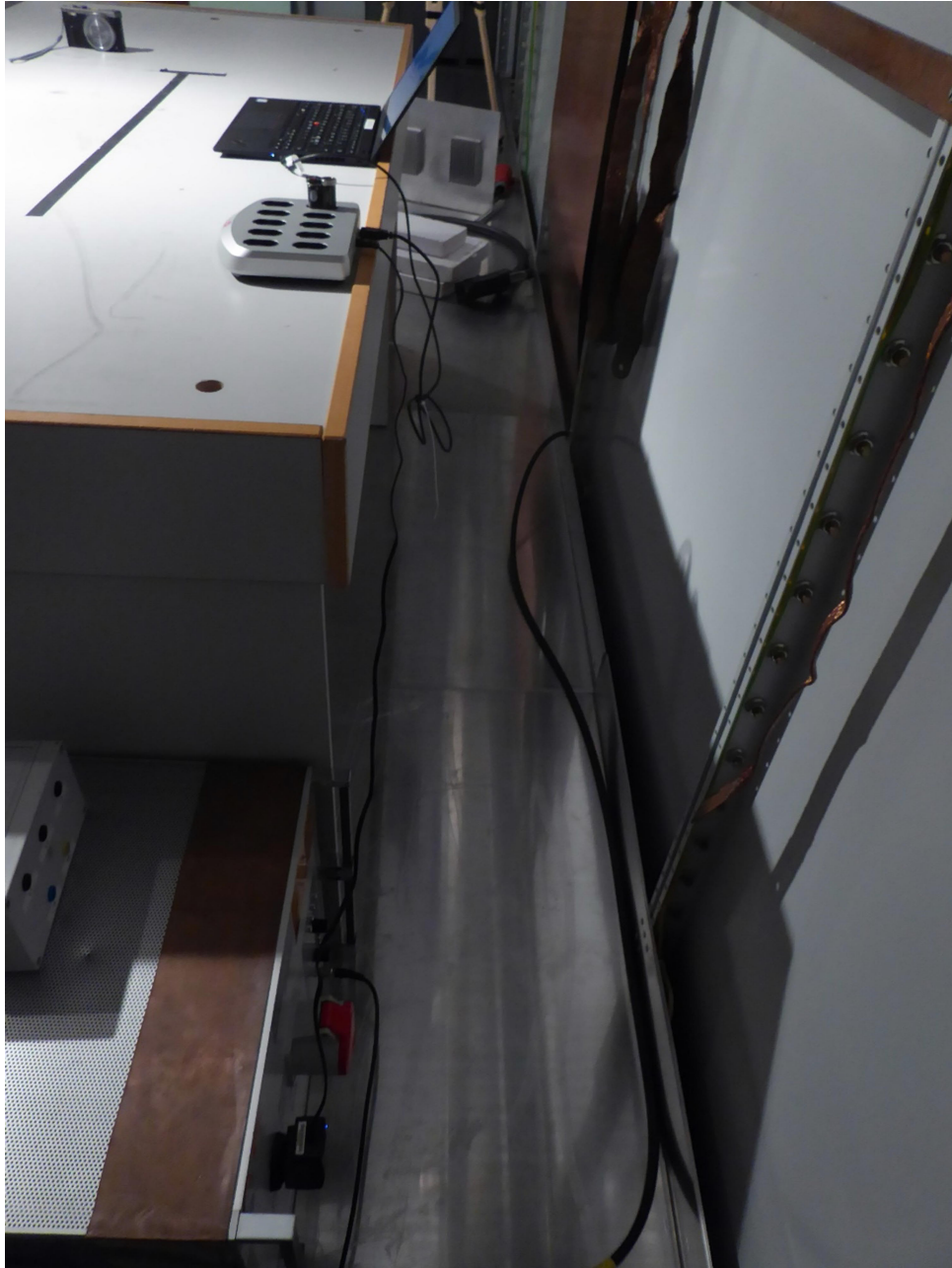
Test setup shielded chamber, EUT supplied via AC/DC power adaptor
