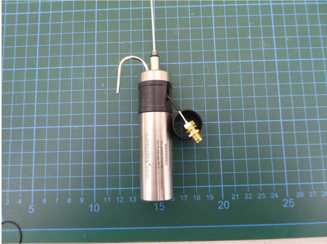
Modification for conducted tests
