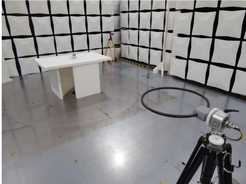
EUT normal orientation (wall mounted) / Antenna Position 3 – ground-parallel Test setup semi-anechoic chamber M276 Preliminary measurement
