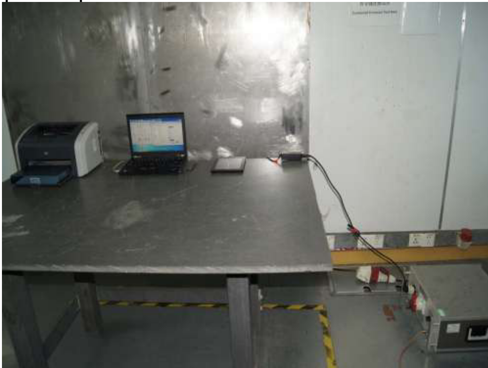
Photograph 2: Set-up for Radiated Emission of below 1GHz
