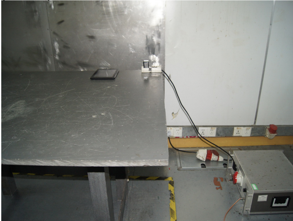
Photograph 2: Set-up for Radiated Emission of below 1GHz
