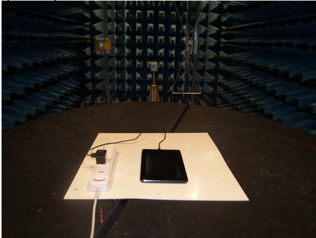
Photograph 5: Set-up for Radiated Emission of 26.5 - 40GHz
