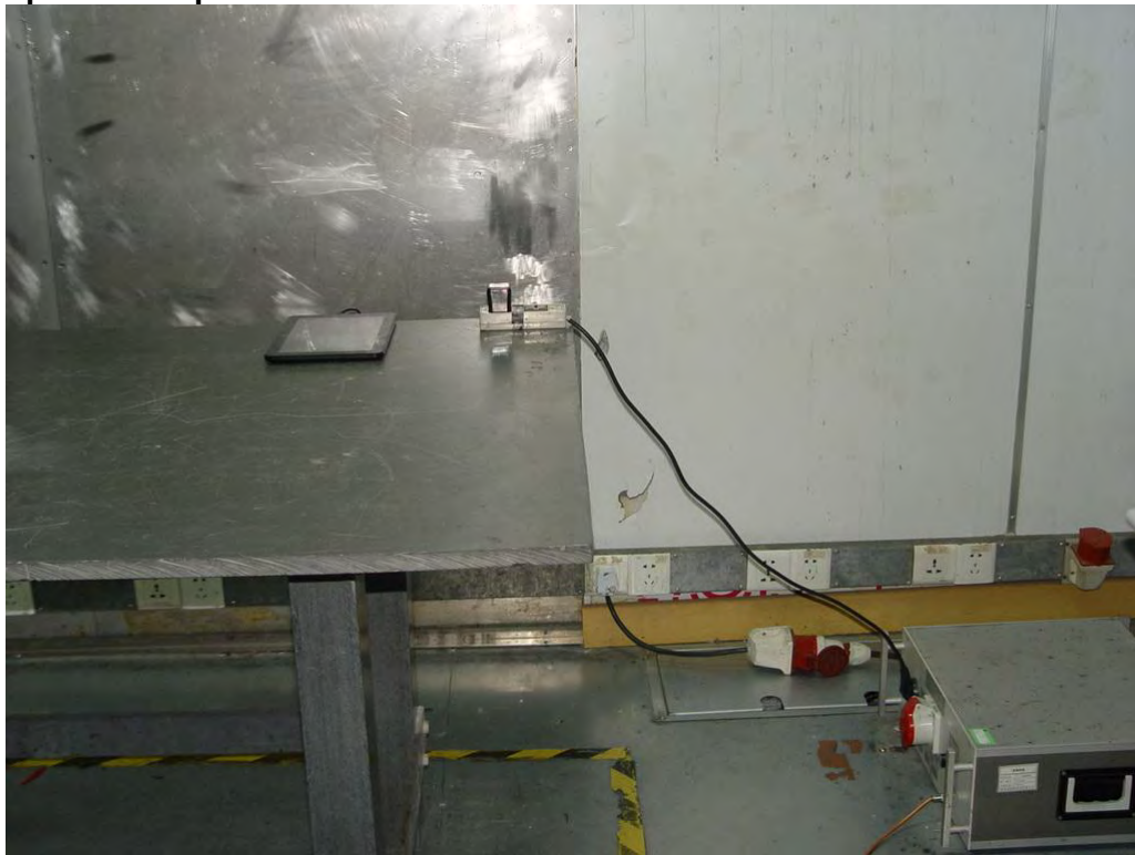
Photograph 1: Set-up for Conducted Emission
