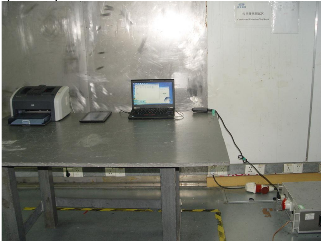
Photograph 2: Set-up for Radiated Emission of below 1GHz
