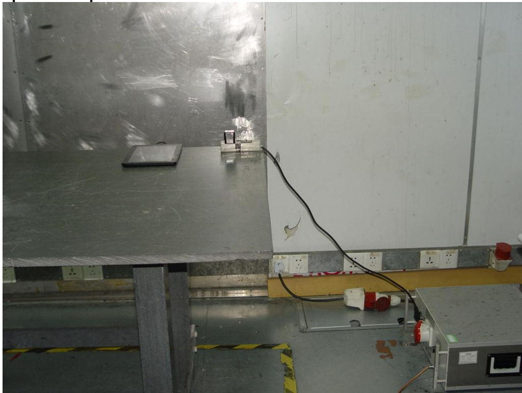
Photograph 1: Set-up for Conducted Emission
