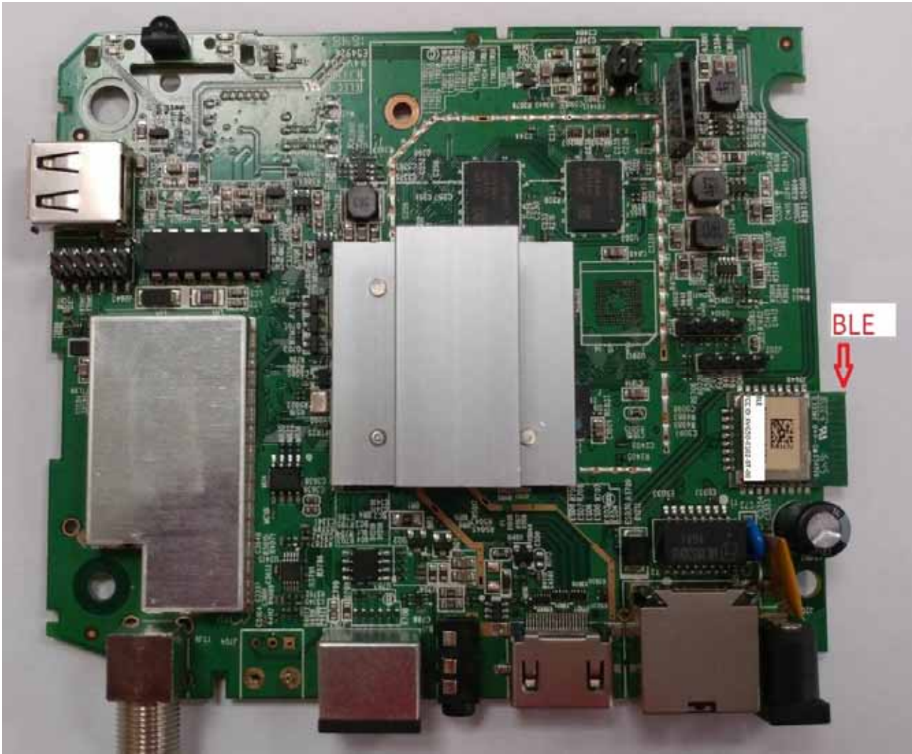
Module install location on Aria6/7.
