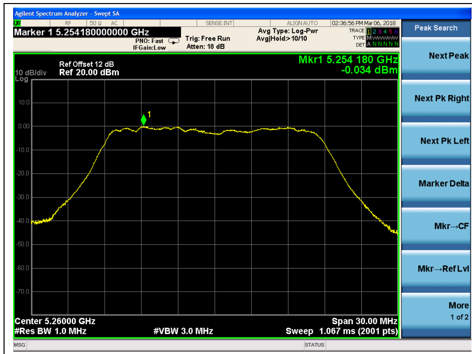
(Channel 52, 5260MHz, 802.11ac (VHT20), ANT J4)
