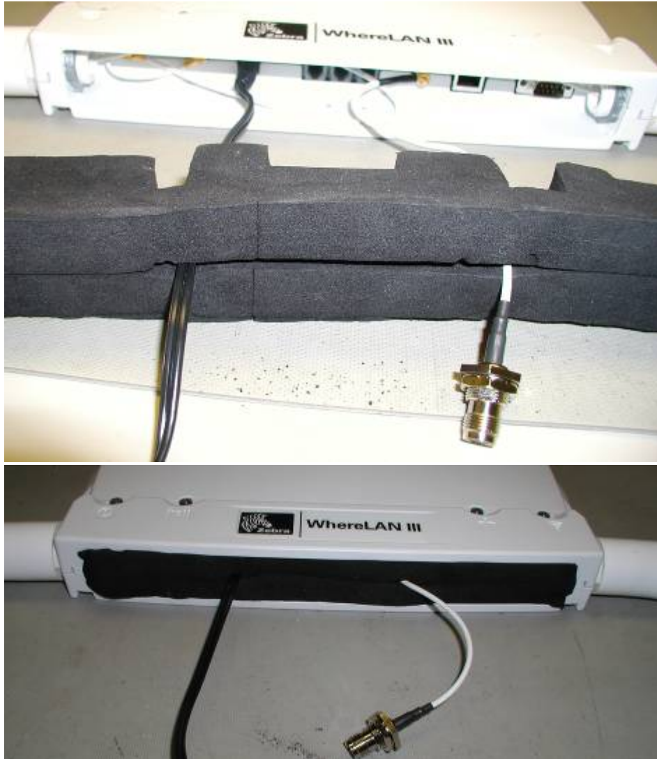
Figure 26 Wi-Fi Cables Drip Plug
