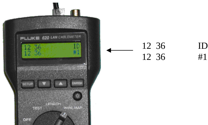
Figure 39 Correct readout when testing 2 pair cable.
