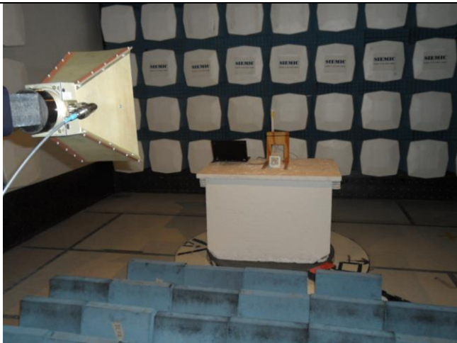
Radiated Emissions (>1GHz) – Front View
