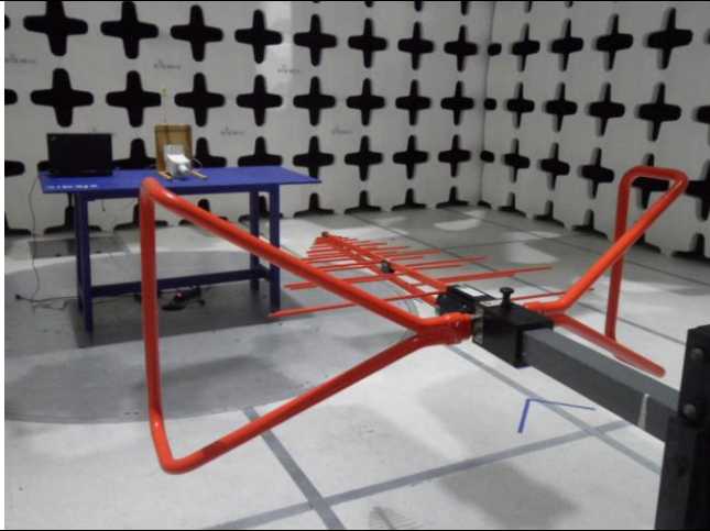
Radiated Emissions (<1GHz) – Front View
