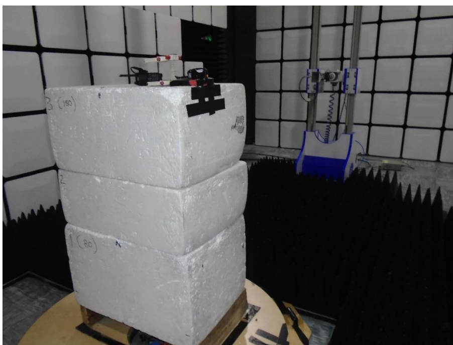
Figure 122 - Test Setup - 1 GHz to 3 GHz Z-Plane
