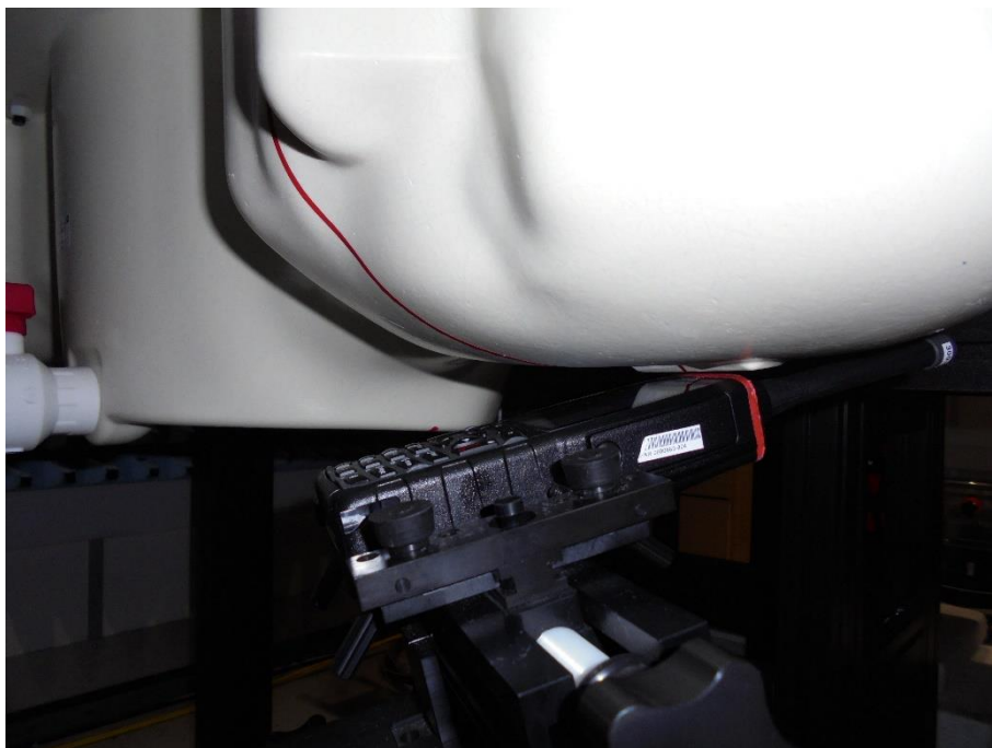
Figure C.2: DUT next to the right ear tilt configuration.
