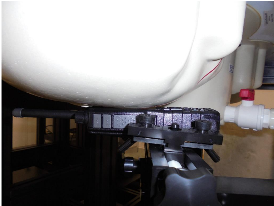
Figure C.3: DUT next to the left ear touch configuration.
