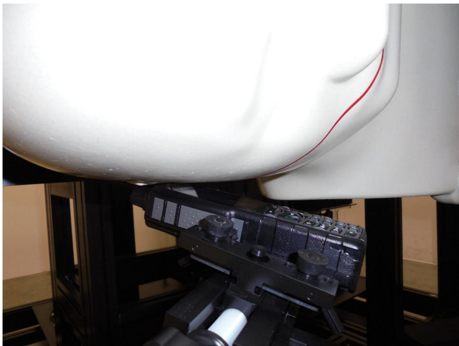
Figure C.4: DUT next to the left ear tilt configuration.
