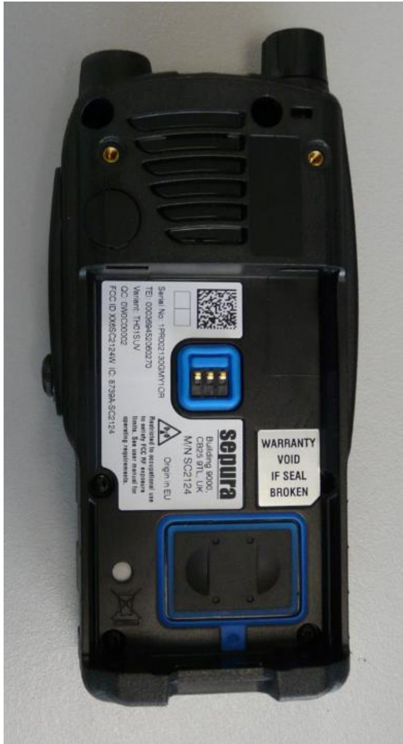
Figure 3. SC21 Series Rear with Battery and Antenna Removed
