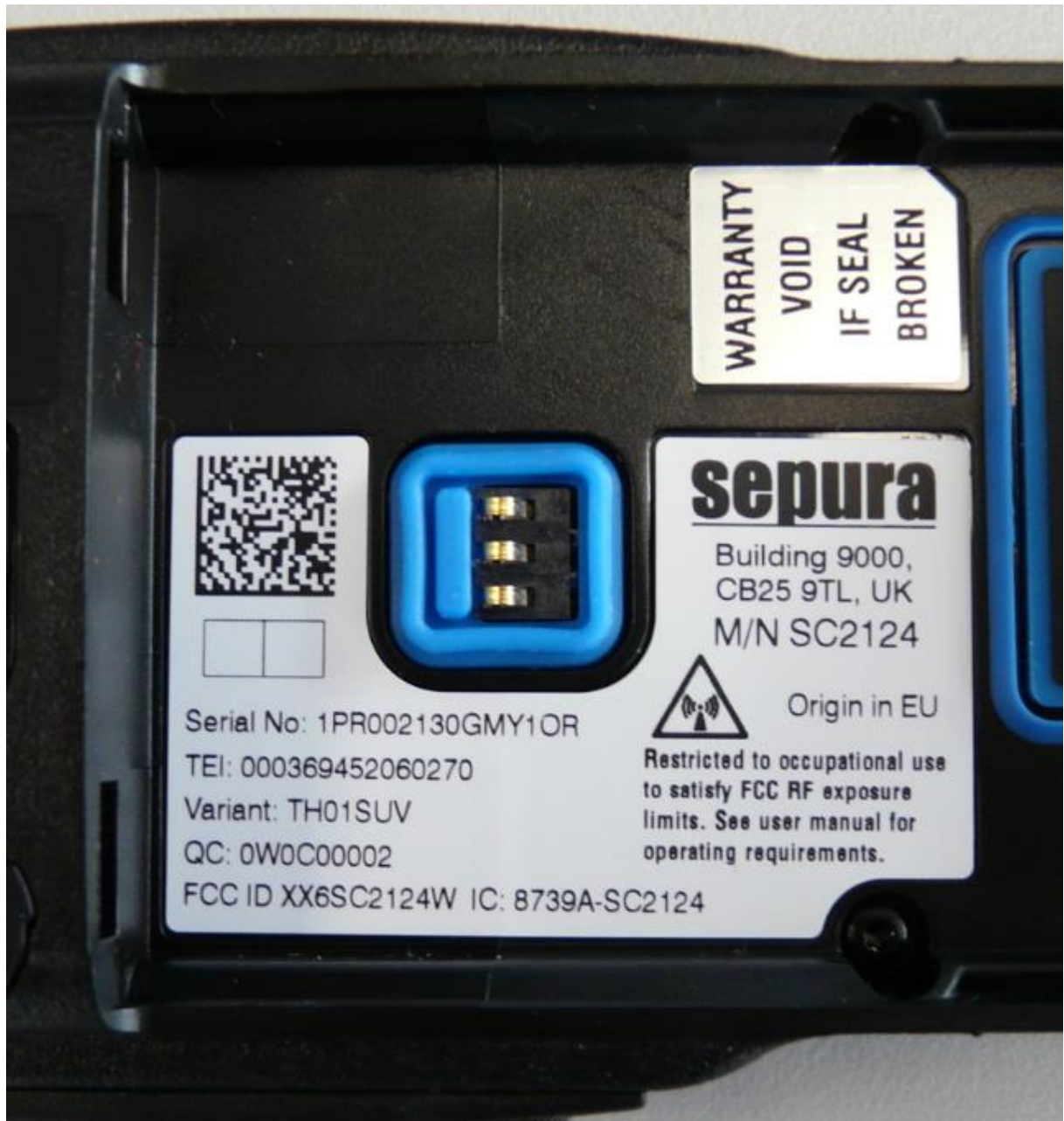
Figure 4. SC21 Series Rear with Battery and Antenna Removed (label closeup)
