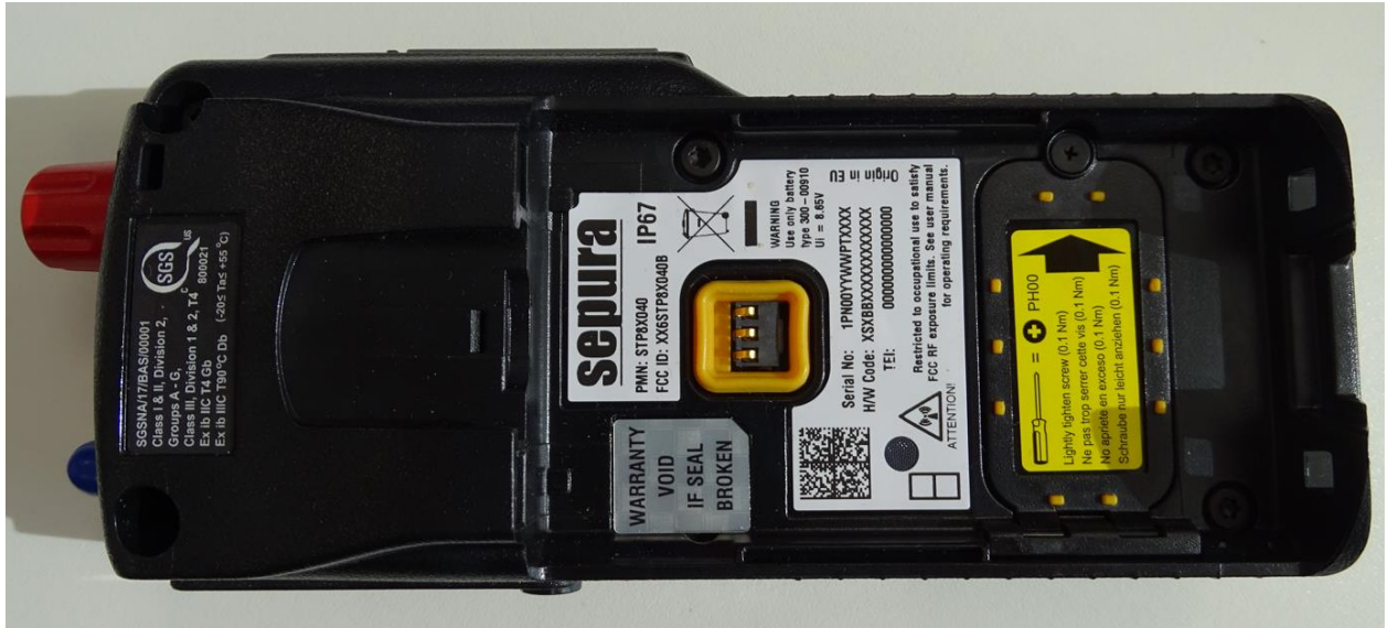
Figure 6. STP8X FCC main label location
