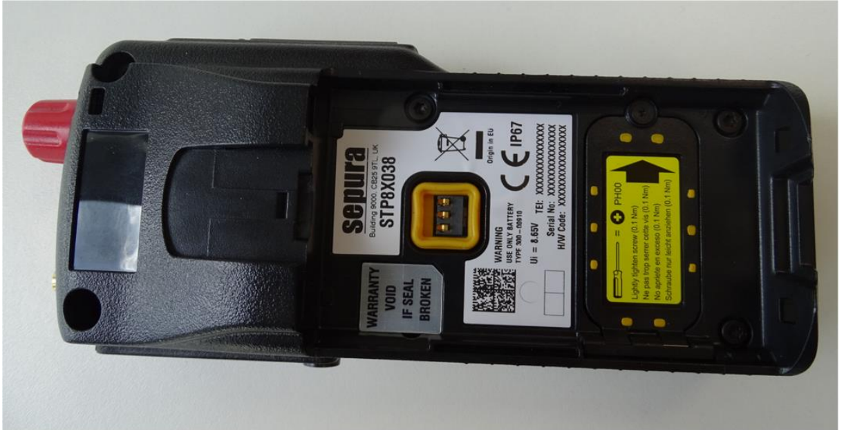
Figure 5. STP8X CE main label location
