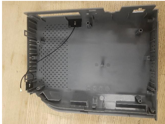
Photograph 10. CNX-WiFi, Internal 5 GHz Antenna Position
