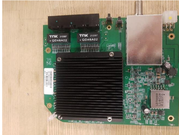
Photograph 7. CNX-WiFi, Internal Board, Side 1
