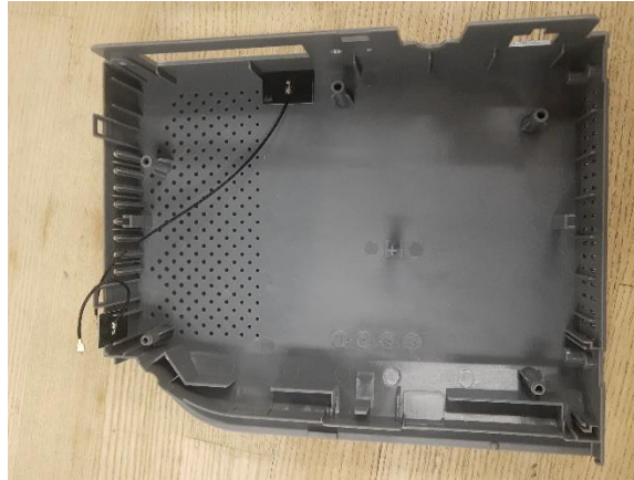
Photograph 10. CNX-WiFi, Internal 5 GHz Antenna Position
