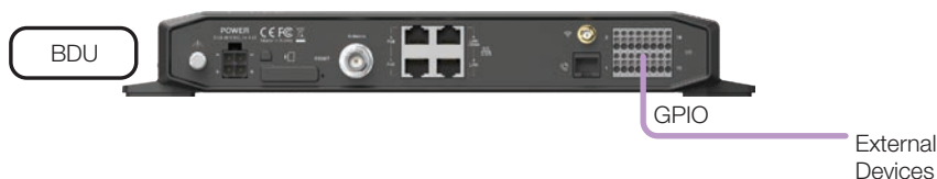
Figure 28: BDU to External Devices Connection
