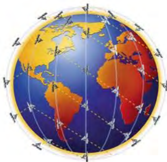
Figure 1: Earth Showing Iridium Satellite in Six Defined Orbital Planes
